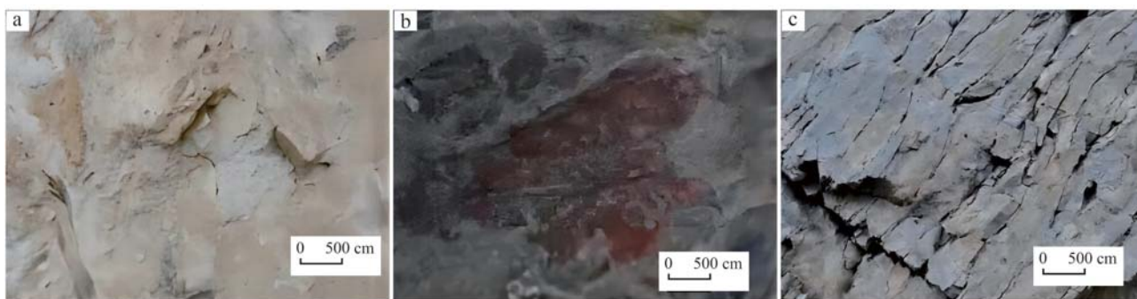
图 6 野外查证获取的各找矿靶区关键围岩蚀变情况 Fig. 6 Alteration of key surrounding rocks in each prospecting target area obtained by field verification a—高岭土化蚀变; b—铁染蚀变; c—碳酸盐化蚀变 a—kaolinization alteration; b—iron stain alteration; c—carbonation alteration
