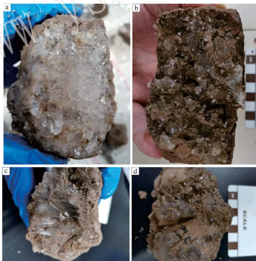
图 10 典型石盐岩储卤层(a,b)和重结晶的巨晶石盐岩(c,d)照片 Fig. 10 Photos of typical halogen reservoir in rock (a, b) and recrystallized macrocrystalline rock (c, d)
