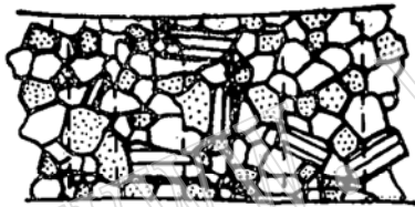
图 1 穿线法统计不同矿物接触数 Fig. 1 Statistics of contact number of different mineral grains by line transection method
